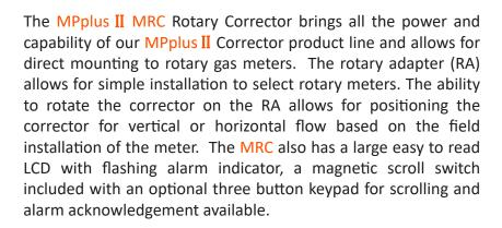
The MPplus II MRC is fully programmable and utilizes dual sockets for onboard communication options, port 2 has two different footprints for the ultimate flexibility in add on IoT modules. Modules consist of cellular radio, RS232, RS485, and many more. A configuration lock out jumper is included to maintain configuration integrity. Four wire RTD provides improved accuracy in temperature measurement.
